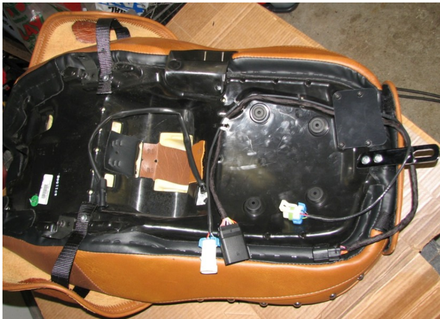
New harness mounted to underside of the seat, parallel to OEM.
