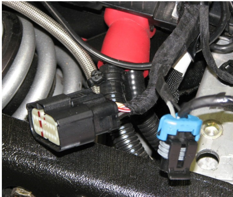
Trunk tail light multi-pin connector on left & accessory 2-pin plug on right.
