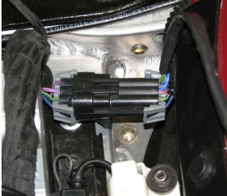
OEM 6-Pin Tail Light connector, under seat, by right side frame.
